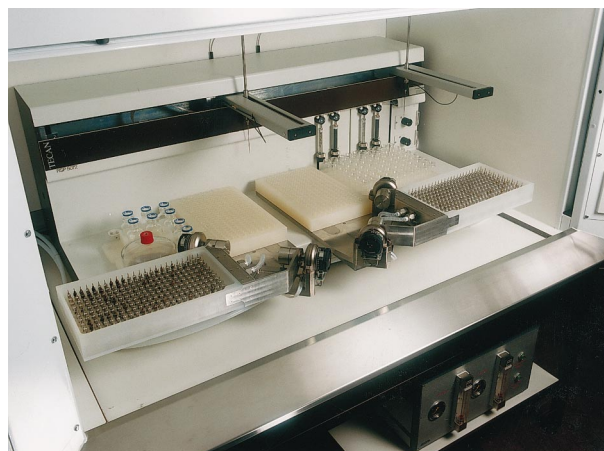
Figure 1. ARNIE, the first solution-phase robotic synthesizer at Glaxo, capable of 480 parallel reactions and solvent removals.
